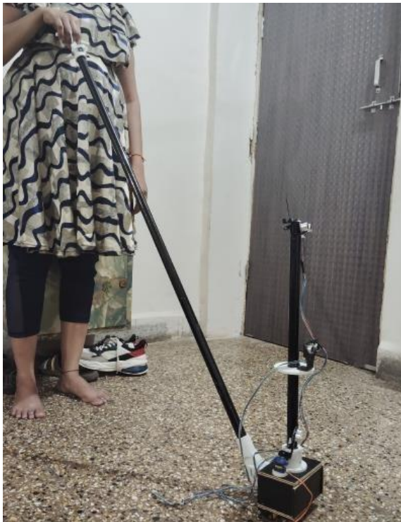
Figure 10. Final Smart Cane Structure
