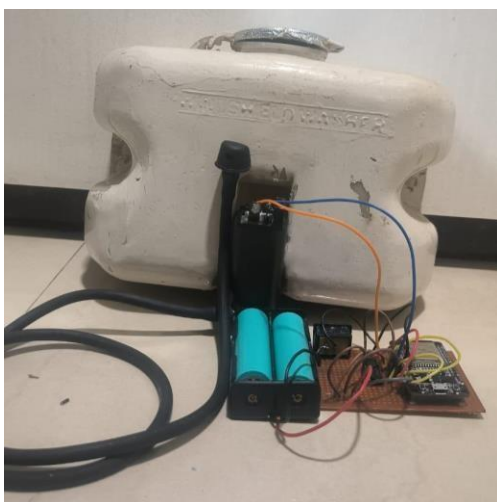
Fig 4. Central system for water supply.
