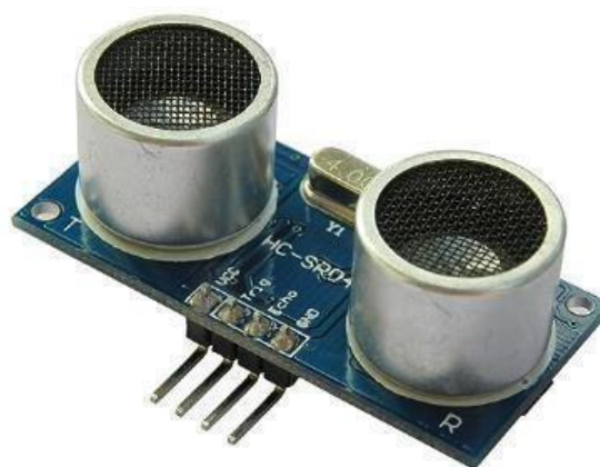
Figure 2. Ultrasonic Sensor (Distance Sensor)
