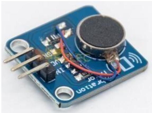
Figure 4. Grove Vibration Motor (Vibration Motor Module)
