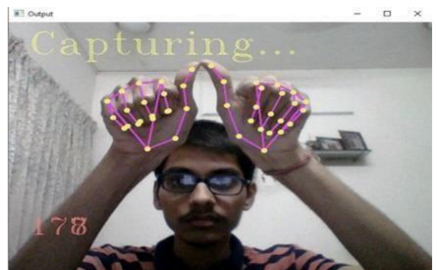
Fig. 3. Using MediaPipe to mark the landmark key points of both hands.
