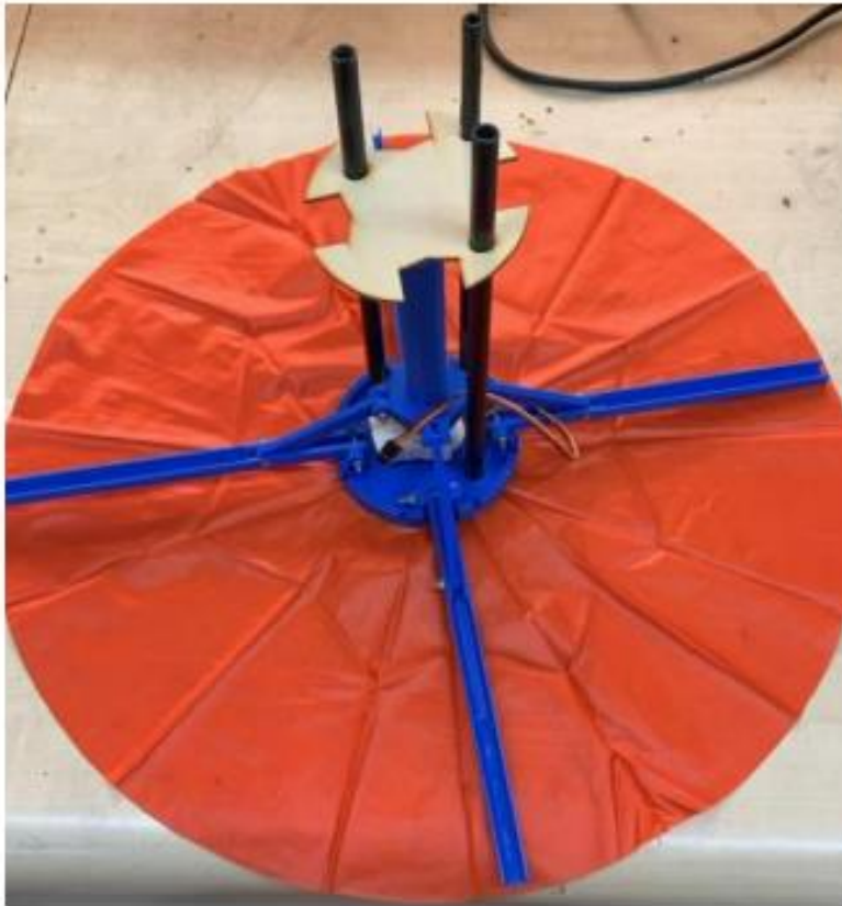
A Skeleton of the Probe module with custom heat shield and carbon fibre rods of the CanSat during the testing before the Critical Design Review
