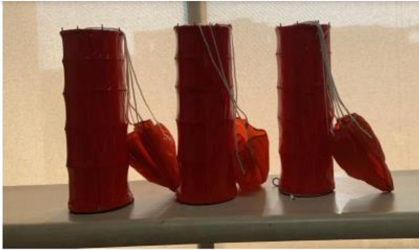
Pictured of the mass manufactured, monokote covered Container for International CanSat Competition 2023
