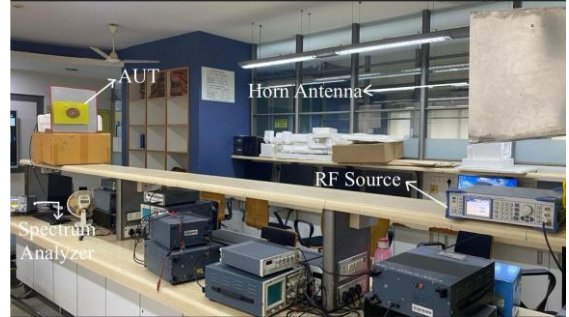
Fig. 7. Broadside Gain Measurement
