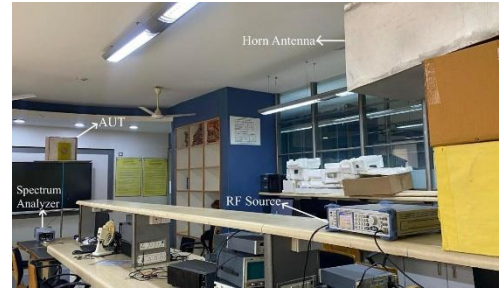
Fig. 6. Radiation Pattern Measurement
