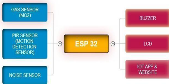
Fig.5 Home Security and Surveillance Security Architecture
