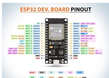
Fig. 1. ESP32 Pinout- detailspin.com
