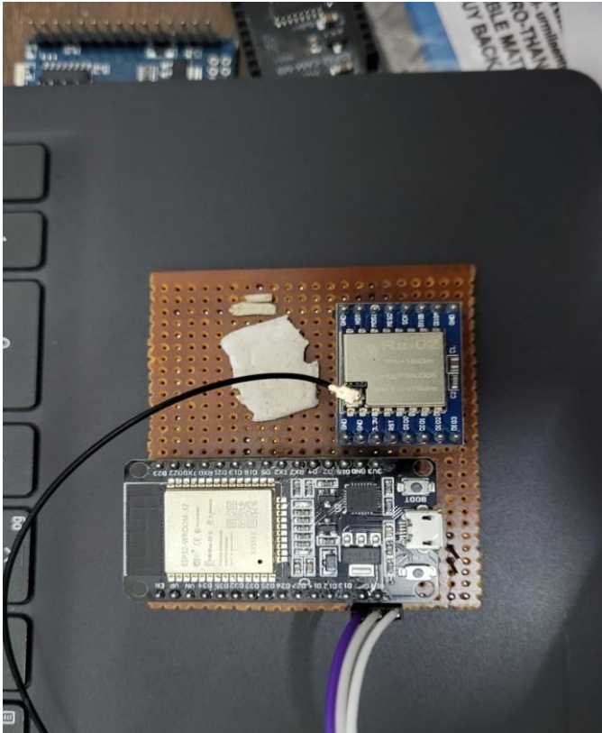
Fig. 2. Hardware Circuit of LoRa-based communication.
